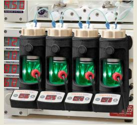
10% to 100% of maximum power, with wavelengths between 365nm and 700nm.
